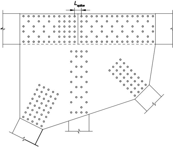
Figure 6A.6.12.6.9-1—Example Connection Showing the Chord Splice Parameter,  $L_{splice}$
