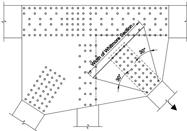
Figure 6A.6.12.6.8-1—Example Connection Showing the Whitmore Section for a Tension Member Derived from 30 Degree Dispersion Angles
