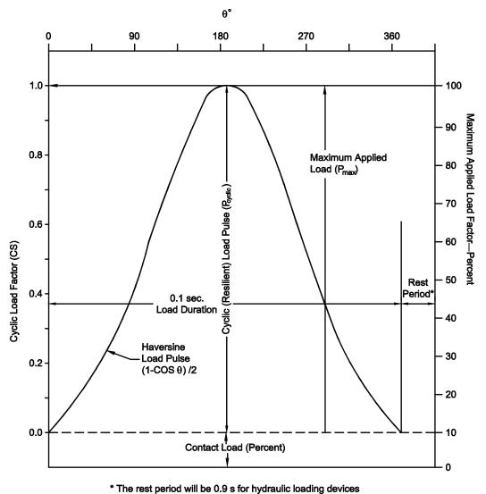
and 0.9 to 3.0 s for pneumatic loading devices.
