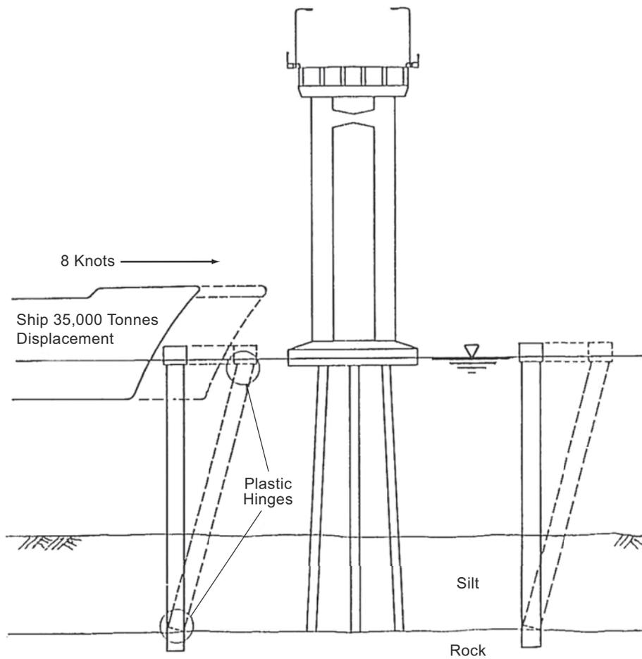
Figure C7.3.2-4—Section of Pile-Supported Pier Protection System Evaluated for the Tasman Bridge
