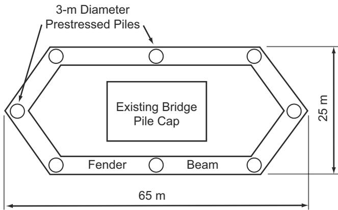
Figure C7.3.2-3—Plan of Pile-Supported Pier Protection System Evaluated for the Tasman Bridge, Australia (All Units Are Metric)
