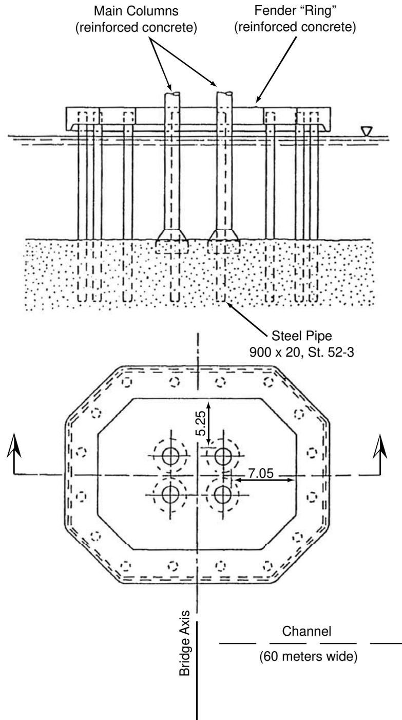
Figure C7.3.2-2—Pile-Supported Protection System for the Tromsø Bridge, Norway (All Units Are Metric)
