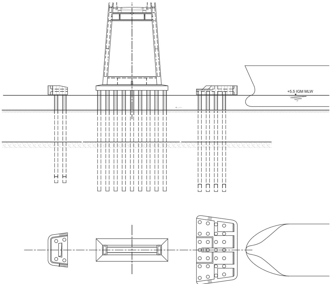
Figure C7.3.2-5—Pile-Supported Protection System for the Rosario-Victoria Bridge, Argentina
