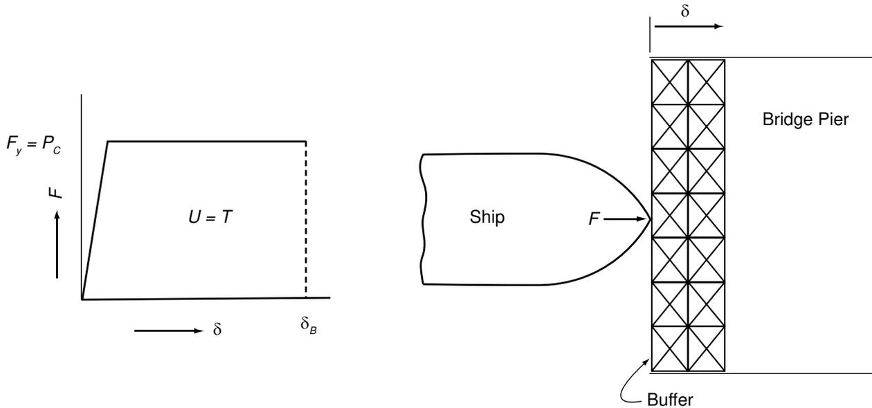
Figure C7.3.1.4-2—Load-Deformation Relationship of Framed Steel Fender Wall
