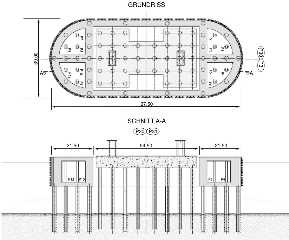
Figure C7.3.2-6—Pile-Supported Protection System for the Orinoco Bridge, Venezuela
