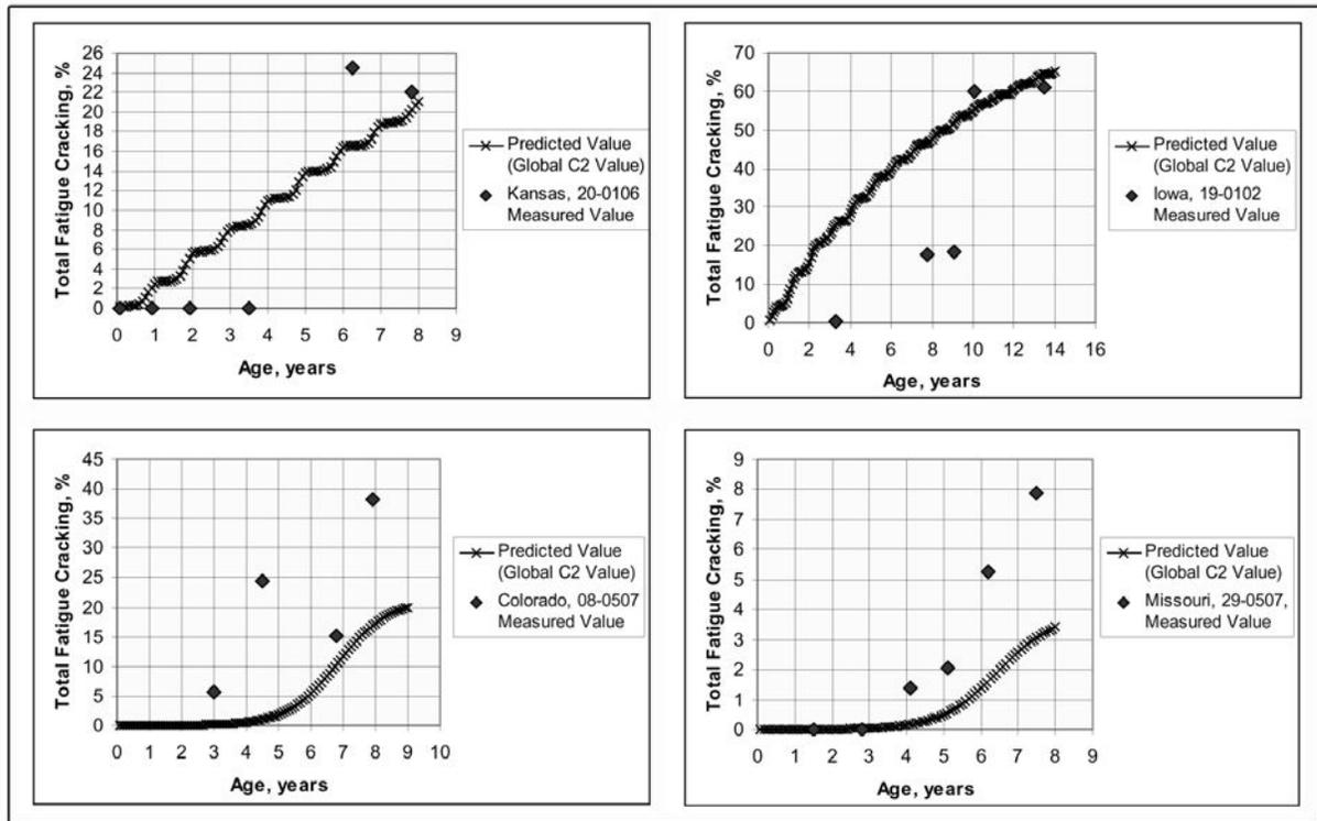
**Figure A2-22. Comparison of Measured and Predicted Values of Fatigue Cracking for Specific Test Sections**
