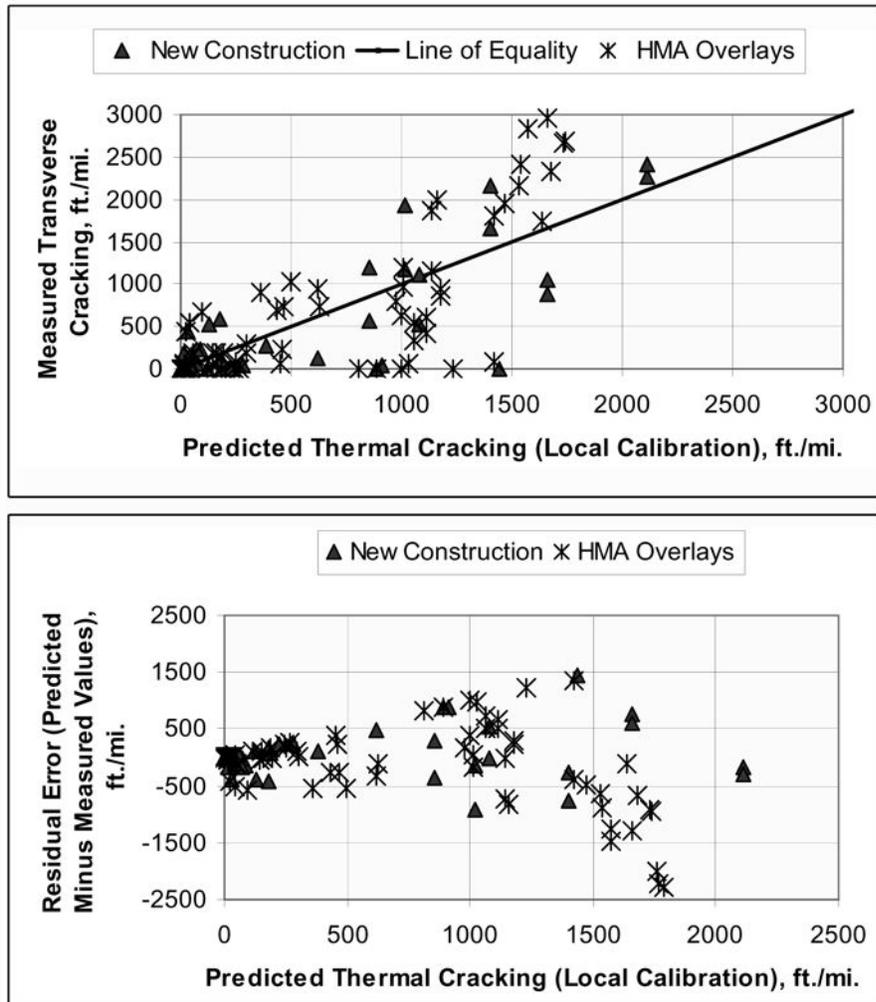
**Figure A2-24. Comparison of Predicted Thermal Cracking and Measured Transverse Cracking Using the Local Calibration Values for the HMA Mixture**
