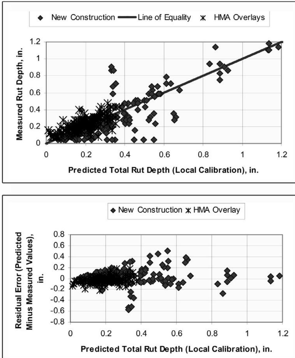
**Figure A2-21. Comparison of Predicted and Measured Rut Depths Using the Local Calibration Values for the Subgrade, Unbound Aggregate, and HMA Layers**
