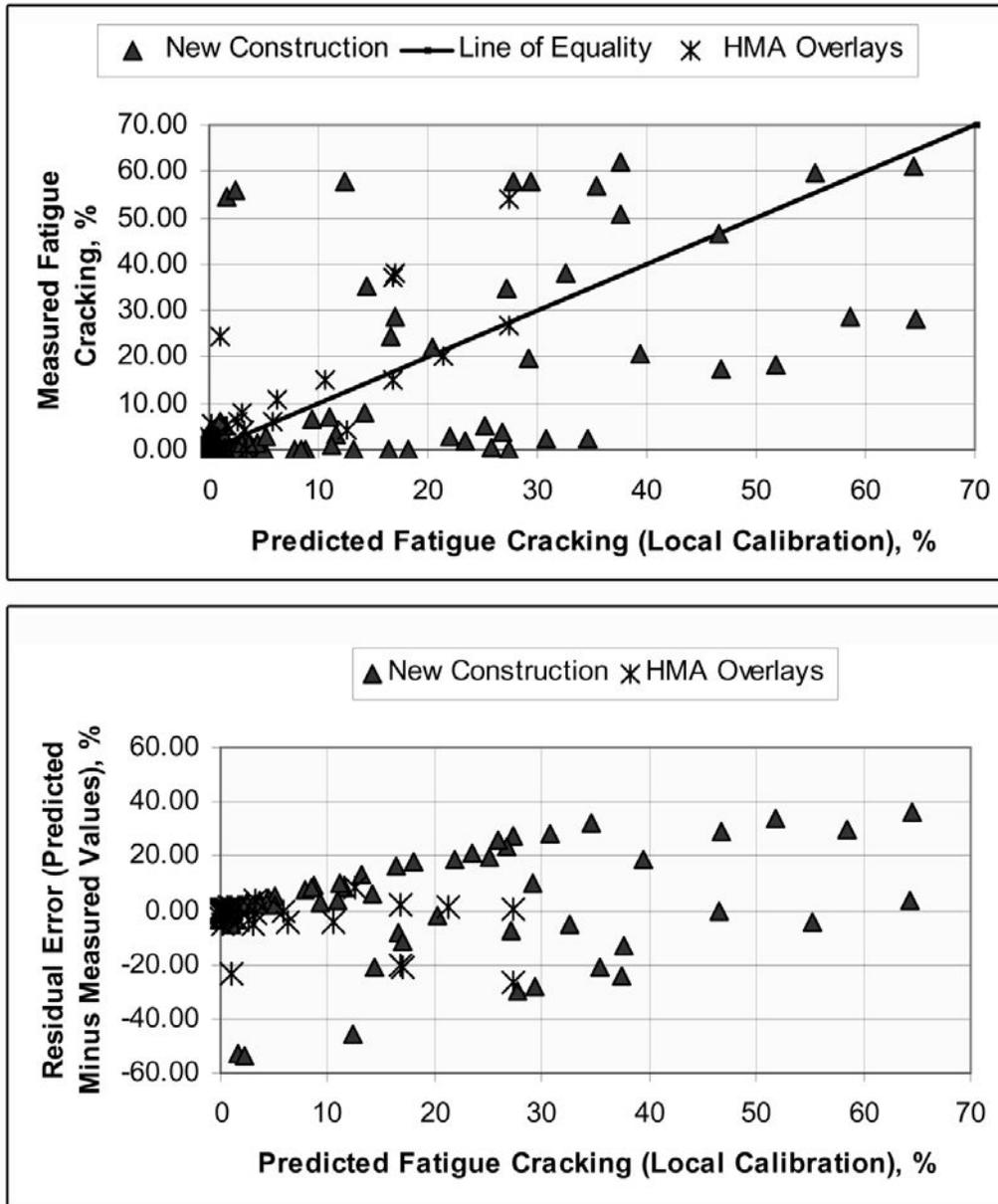
**Figure A2-23. Comparison of Predicted and Measured Fatigue Cracking Using a Local Calibration Value for the HMA Mixture That Is Air Void Dependent**
