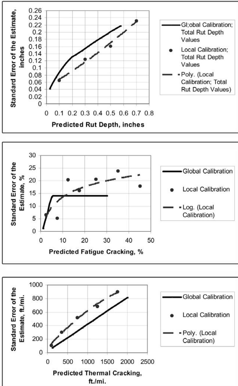
**Figure A2-26. Comparison of the Standard Error of the Estimate from the Global and Local Calibration Process**
