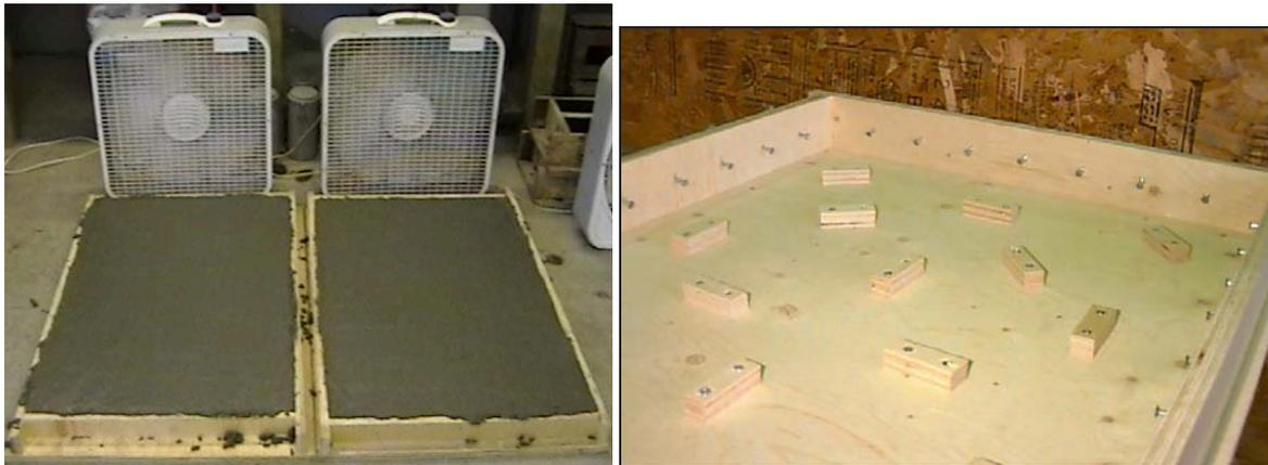
Figure 3. Plastic Shrinkage Panel Configuration and Internal Restraints
