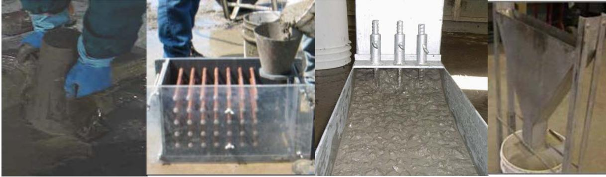
Figure 2. From left to right (Slump Flow, Filling Capacity, L-Box and V-Funnel)
