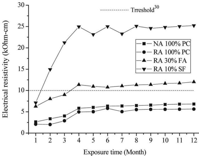
Fig. 5—Evolution of electrical resistivity as a function of exposure time
