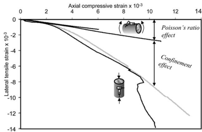
Fig. 9.10—Comparison between axial-lateral strain behavior in beams and columns (Fam and Rizkalla 2002).
