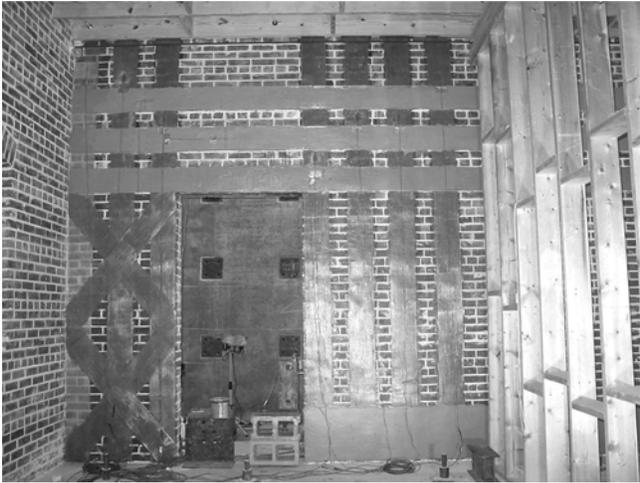
Fig. 10.1—Precured structural grids embedded in trowel-applied epoxy adhesive (Moon 2004).
