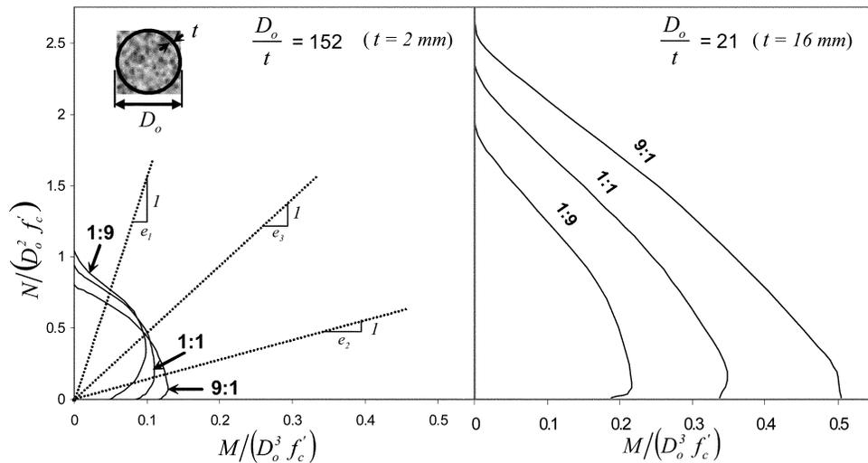
Fig. 9.12—Effect of thickness and laminate structure of tubes on interaction curves of CFFT (Fam et al. 2003b).
