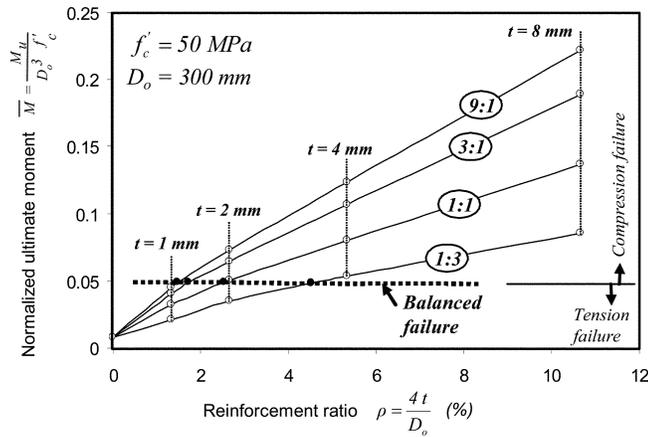
Fig. 9.9—Variation of flexural strength with reinforcement ratio for different laminate structures (Fam and Rizkalla 2002.)
