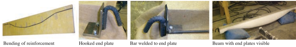
Figure 5 — Anchorage using welded end plates.
