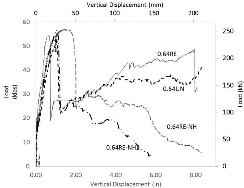
Figure 8- Post punching of anchored and unanchored tensile reinforced slabs
