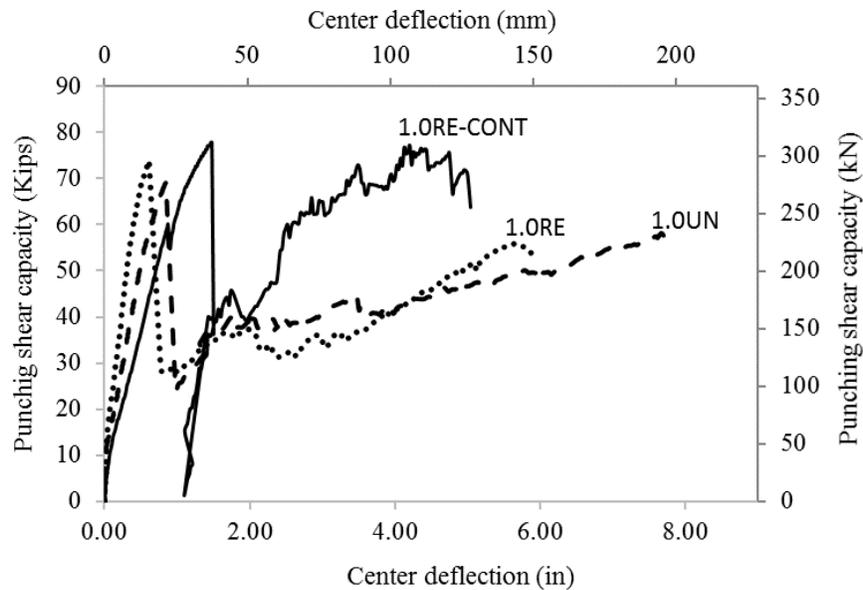
Figure 11- Effects of slab integrity reinforcement on post-punching capacity.
