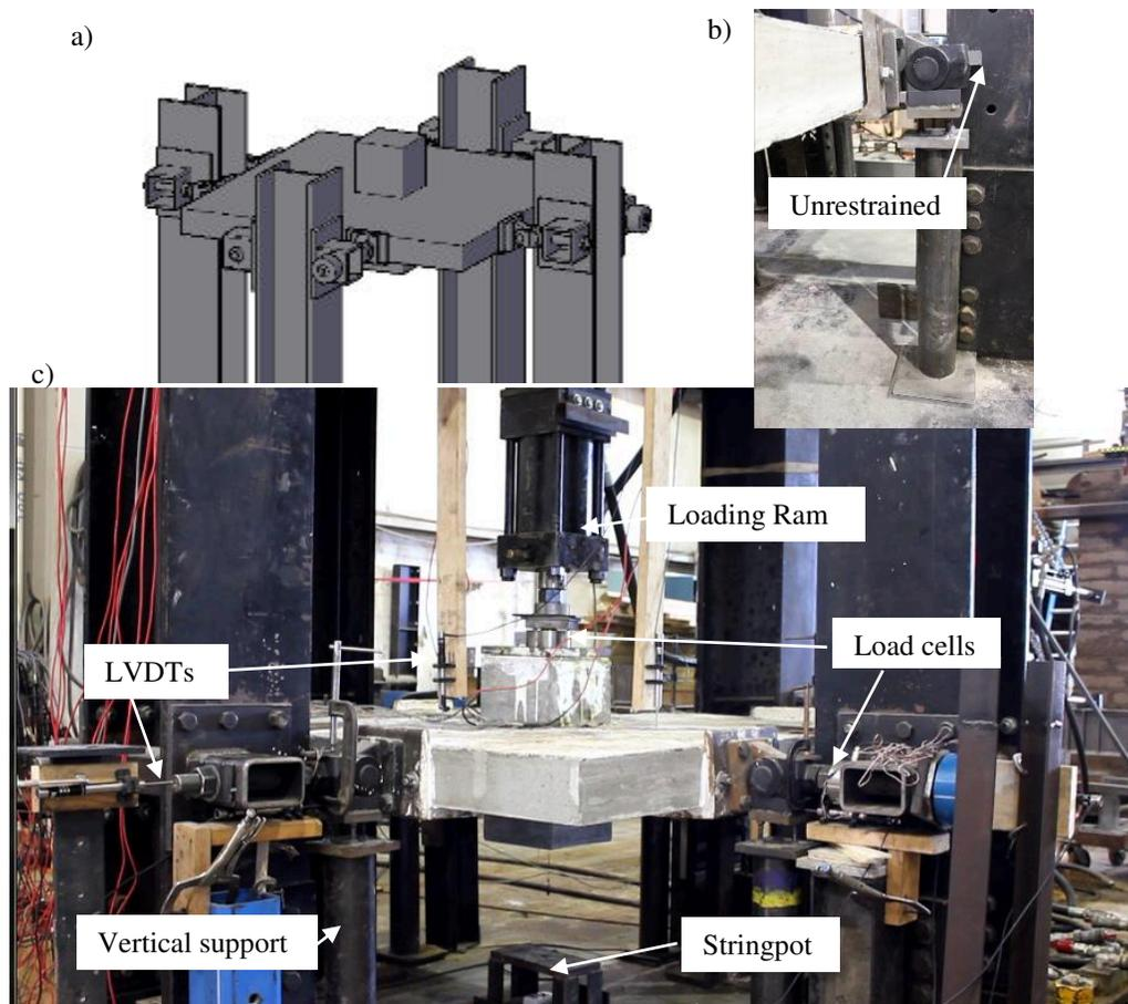
Figure 6 – Test setup: (a) test schematic, (b) support for specimens without lateral restraint, and (c) test setup and instrumentation of restrained specimens.
