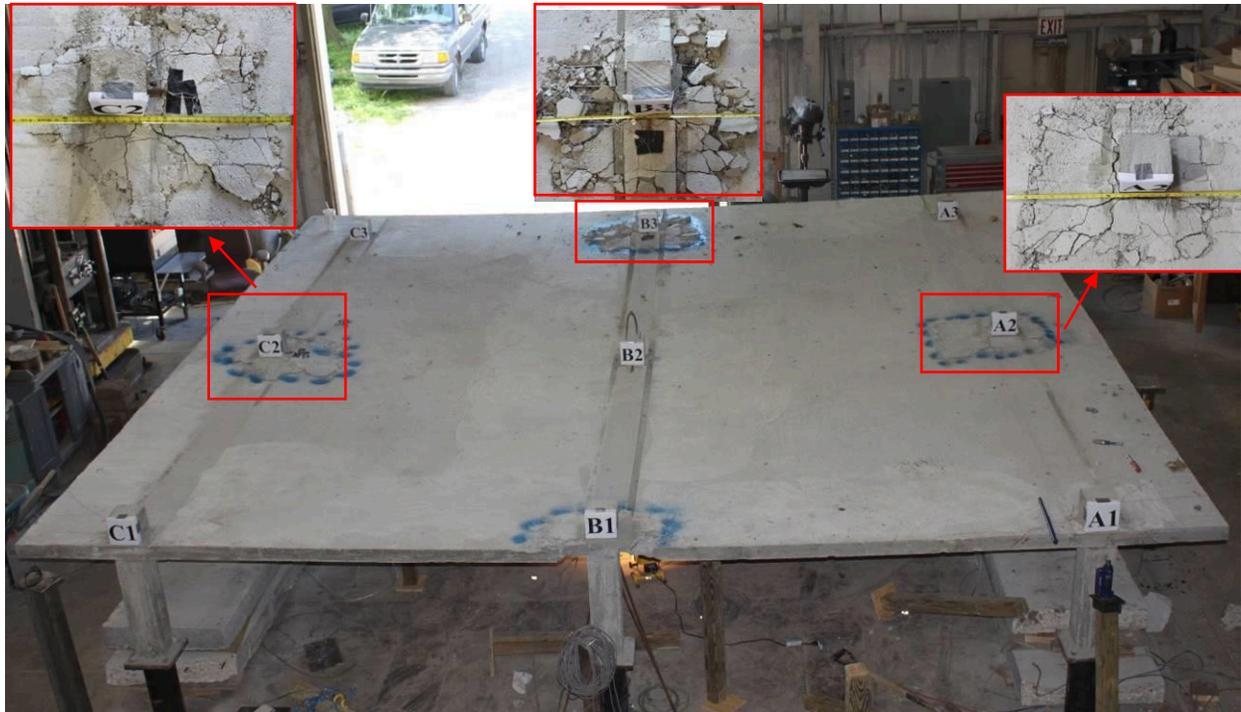
Figure 3 – Multi-panel flat plate specimens without progressive collapse due to post-punching resistance of slab-column connections (Peng 2015).
