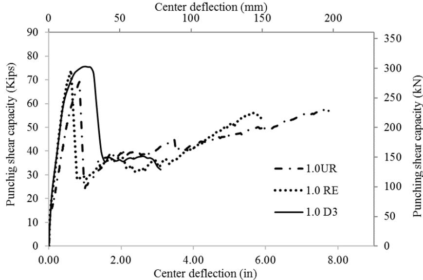
Figure 10- Comparisons of post-punching capacity between static and dynamic tests.
