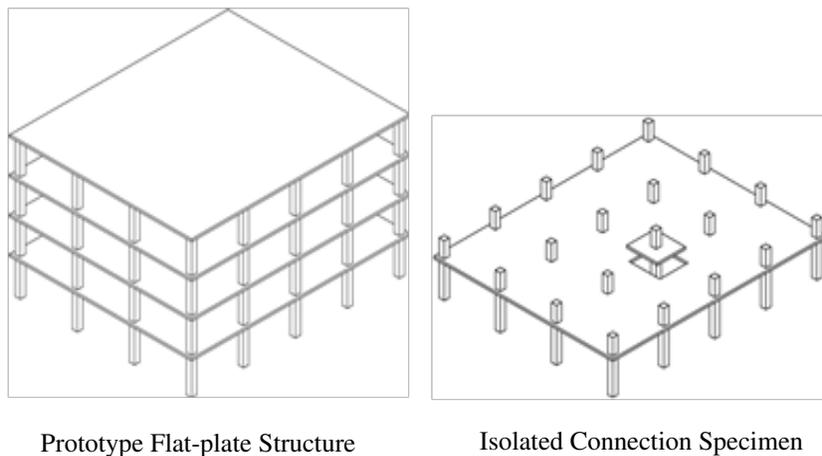
Figure 4- The relationship between tested specimens and prototype
