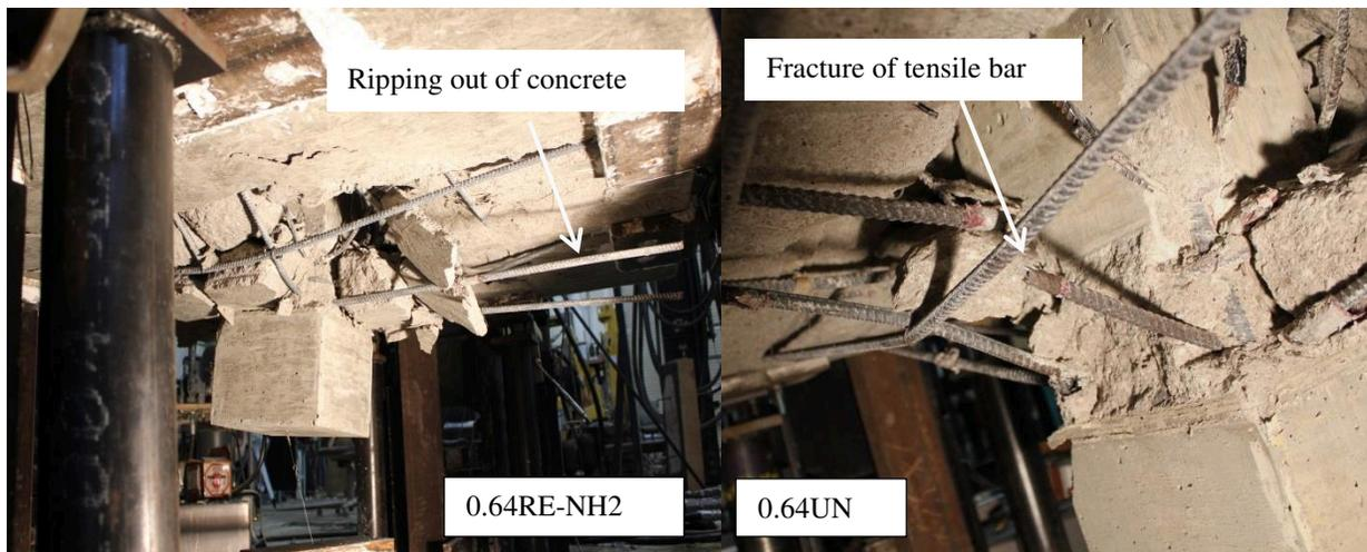
Figure 9- Post-punching failure modes: 0.64RE-NH2 without anchored bars and 0.64UN with anchored bars.
