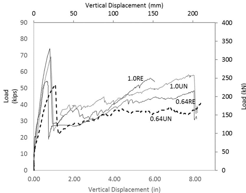
Figure 7 - Effects of reinforcement ratio on post-punching capacity.
