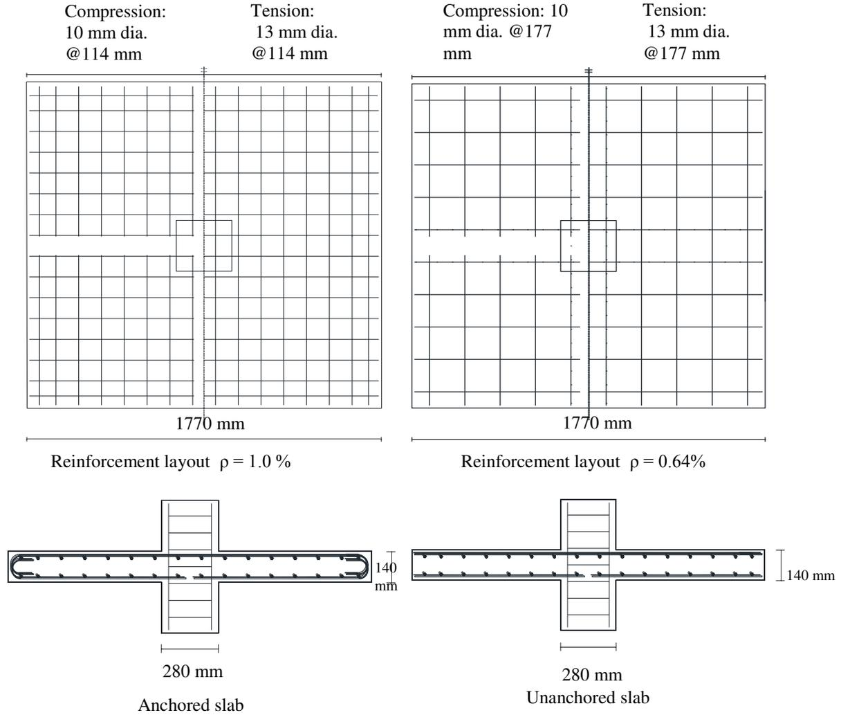
Figure 5 - Dimension and reinforcement layout of specimens
