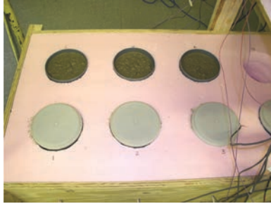
Figure 5—Example of equipment used to measure setting time by monitoring temperature rise.
