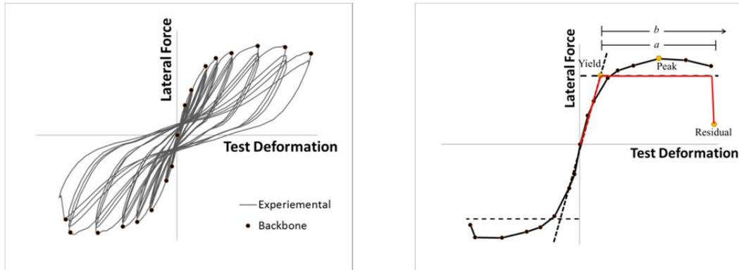
**Figure 3 – Backbone curve generated from experimental data**
