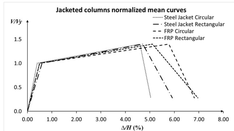
**Figure 4 – Mean force-deformation relationships of jacketed columns from database**
