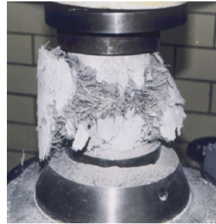
Figure 2 – No fiber concrete cylinder break Figure 3 – FRC extended cylinder break
