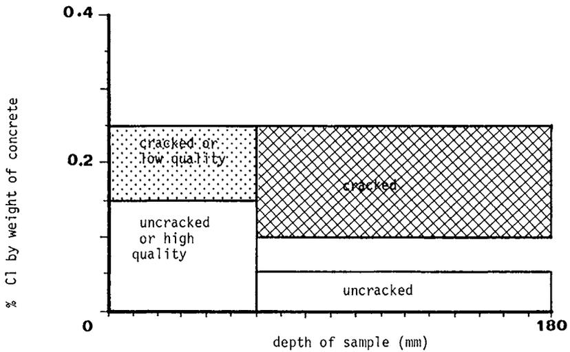
FIGURE 9(b) Chloride penetration into concrete in saline atmosphere, splash or tidal zones
