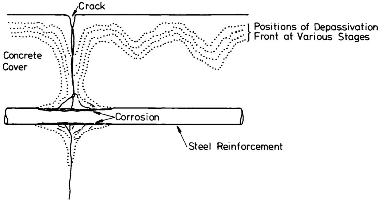
FIGURE 8 Penetration of depassivation fronts at cracks in concrete
