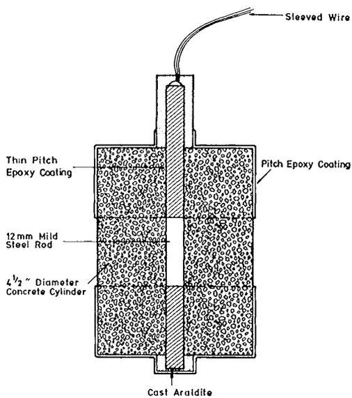
TEST SPECIMEN - REINFORCING STEEL IN CONCRETE
