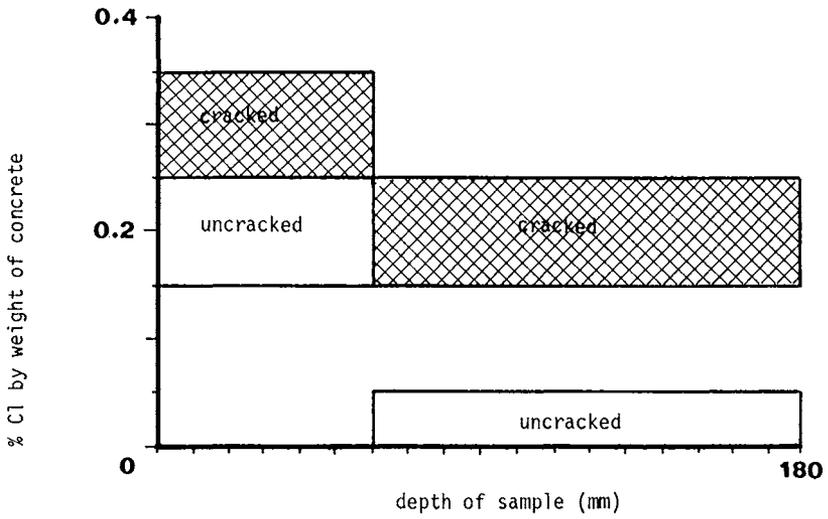
FIGURE 9(a) Chloride penetration into concrete fully submerged in sea water
