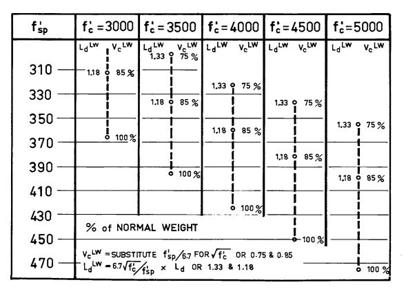
Fig. 6-2-Proposed revision to ACI 318-63, anchorage length and shear
