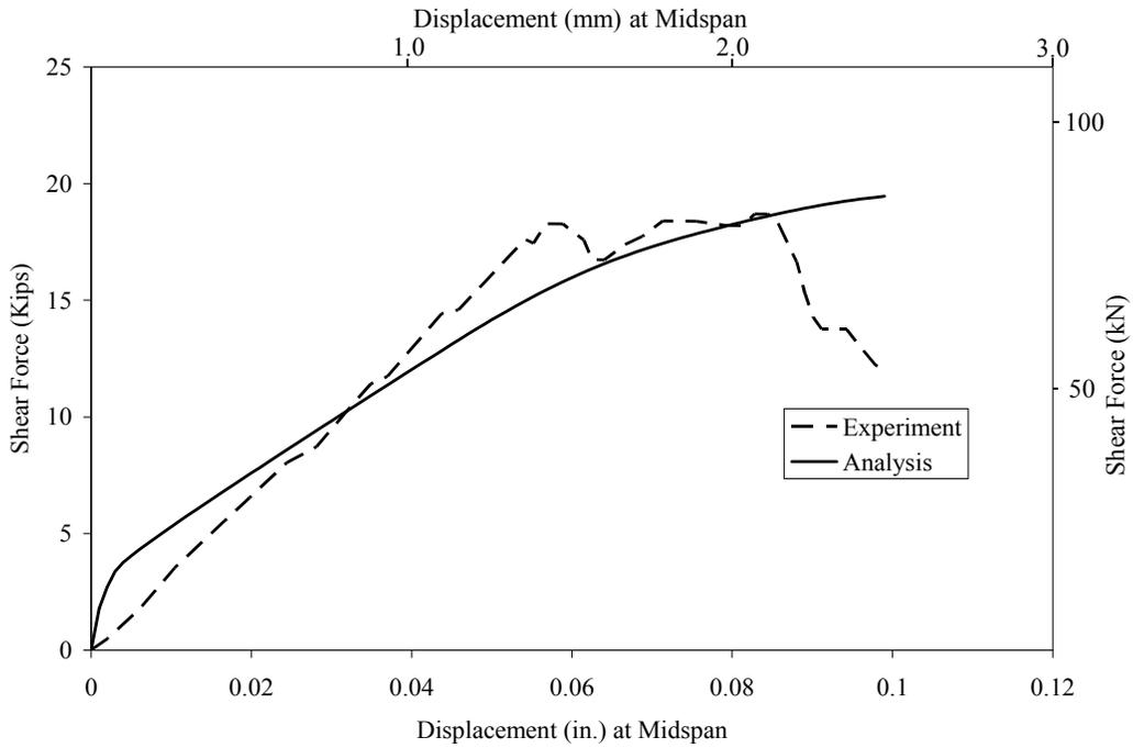
Figure 9 – Shear Force - Midspan Deflection for Beam Z31-FC
