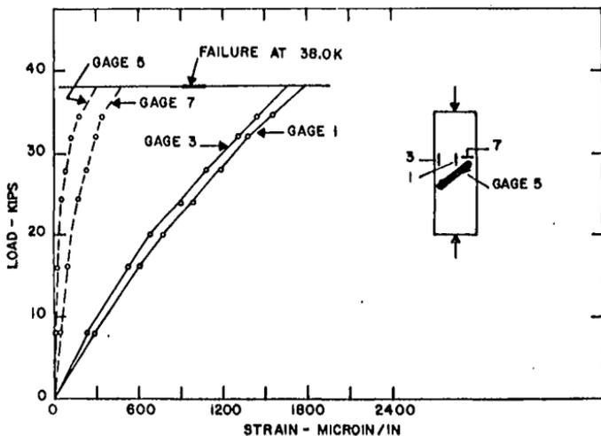
Figure 1-5 Load-strain relations for specimen W-11,  $\phi = 50 \text{ deg}$
