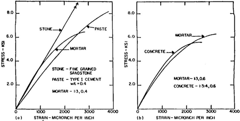
Figure 1-1 Compression stress-strain diagrams for stone, paste, mortar and concrete
