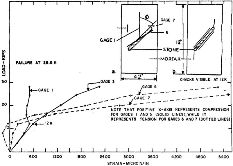
Figure 1-3 Behavior of restrained interface. Specimen, cracks and strains for  $\phi = 23$  deg
