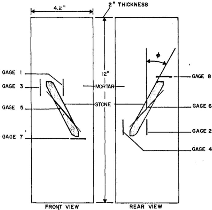
Figure 1-2 The specimen for the interfacial study
