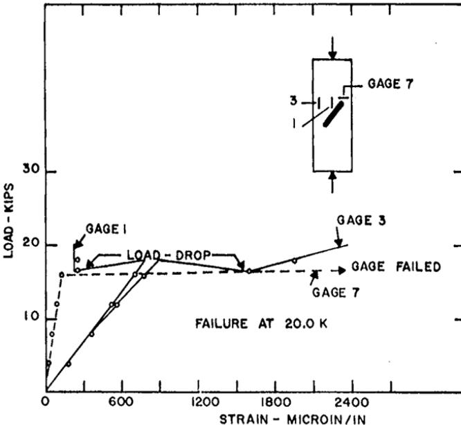
Figure 1-4 Load-strain relations for specimen W-8,  $\phi = 42$  deg
