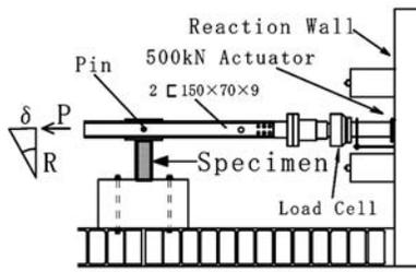
Figure 4 -- Test Setup
