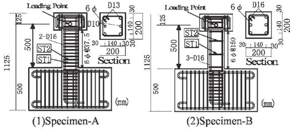
Figure 3 -- Geometry and Reinforcing Arrangement
