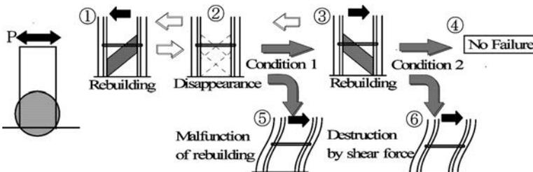
Figure 2 -- Flexural Shear Failure Mechanism in Hinge Region
