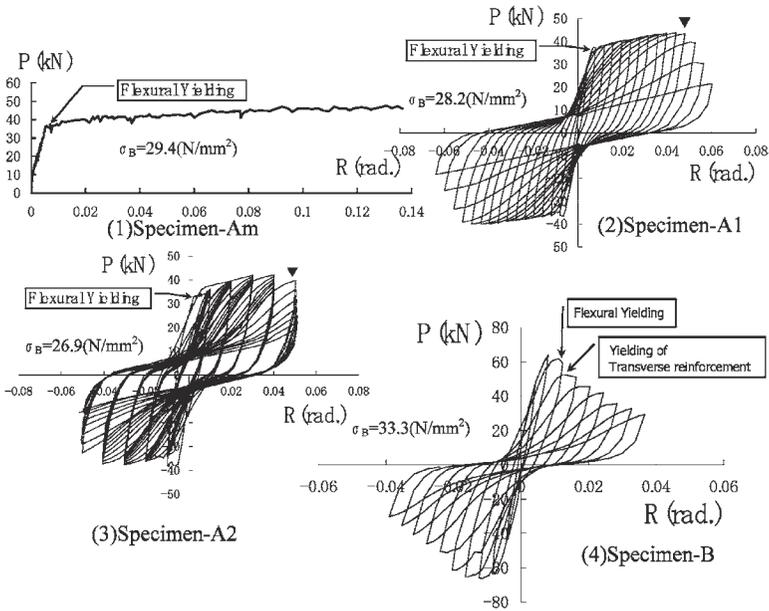
Figure 7 -- Load (P) vs. Drift ratio (R) Relation
