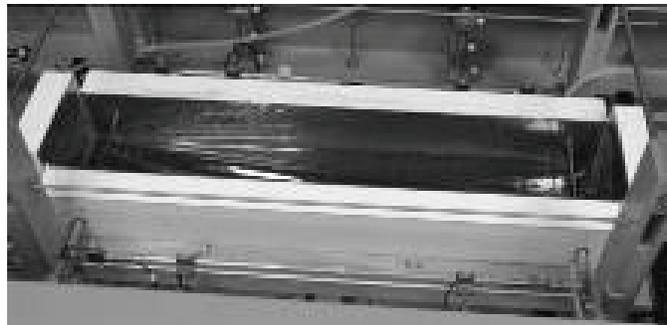
**4a: ADTM setup for autogenous shrinkage testing.**
