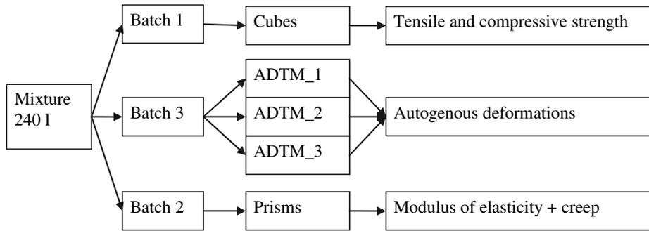
**Figure 2—Schematic representation of the testing program.**
