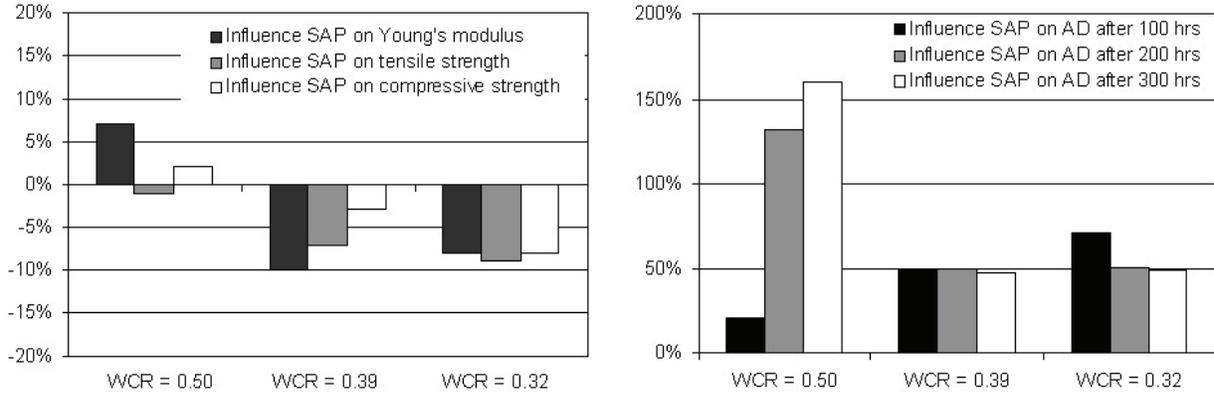
**Figure 6—Left: Influence of SAP (1.5 kg/m<sup>3</sup>) on Elastic modulus, tensile and compressive strength after 28 days of hardening; Right: Influence of SAP (1.5 kg/m<sup>3</sup>) on autogenous shrinkage at three different ages, 100, 200 and 300 hrs respectively. Note: values larger than 100% means swelling of the specimen (see wcr = 0.50).**
