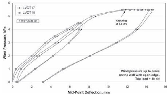
Fig. 9: Cyclic wind load tests up to failure (open edge)
