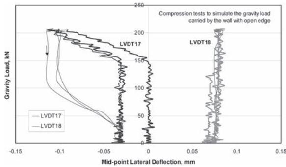
Fig. 8: Cyclic gravity load tests (open edge)
