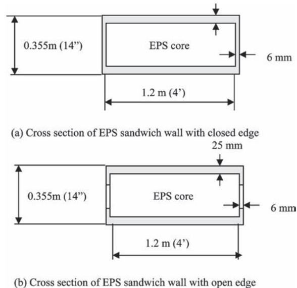
Fig. 1: Cross section of EPS sandwich wall
