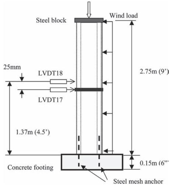
Fig. 2: Side view of sandwich wall (wall thickness = 0.355m)
