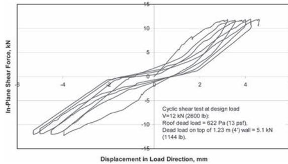
Fig. 7: Cyclic in-plane shear tests (Closed edge)
