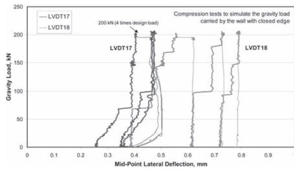
Fig. 5: Cyclic gravity load tests (closed edge)
