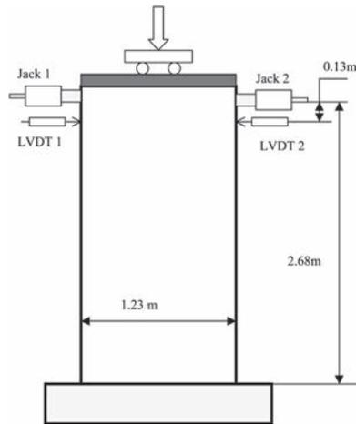
Fig. 4: Front view of sandwich wall
