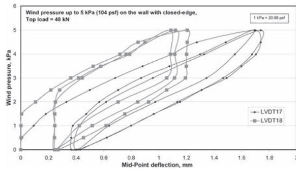
Fig. 6: Cyclic wind load tests (closed edge)
