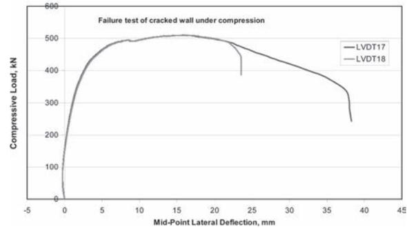
Fig. 10: Failure test of cracked wall up to buckling (open edge)
