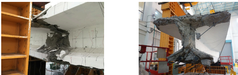
Fig. 13 — Failure of the girder specimens
