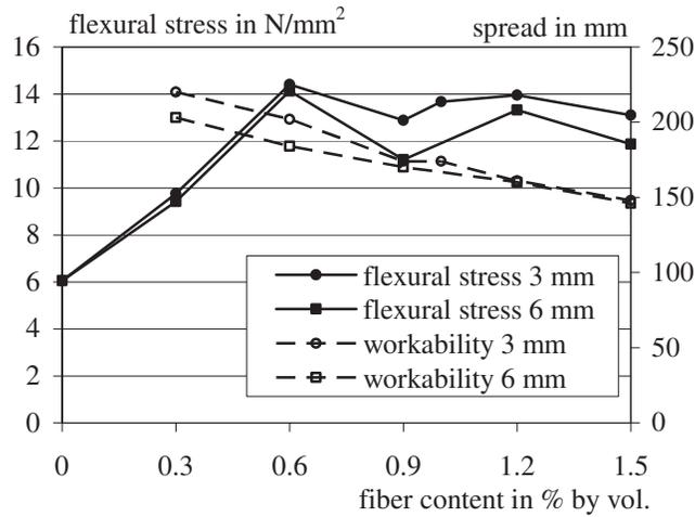
Fig. 4.2 – Influence of fiber content and fiber length on the flexural strength and the workability of concrete containing carbon fibers.
