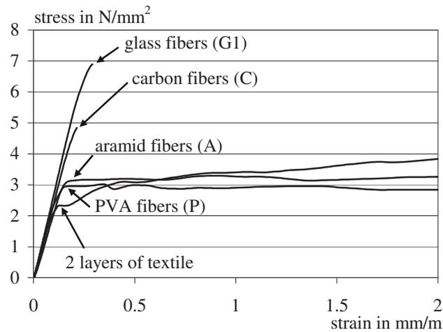
Fig. 4.1 – First crack stresses of specimens with different short fiber types. (1 N/mm<sup>2</sup> = 0.14504 ksi, 1 mm/m = 1 ‰)
