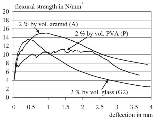
Fig. 4.3 – Post-cracking behavior of flat prisms with different macro fibers in bending tests. (1 N/mm<sup>2</sup> = 0.14504 ksi, 1 mm = 3.937 · 10<sup>-2</sup> in.)
