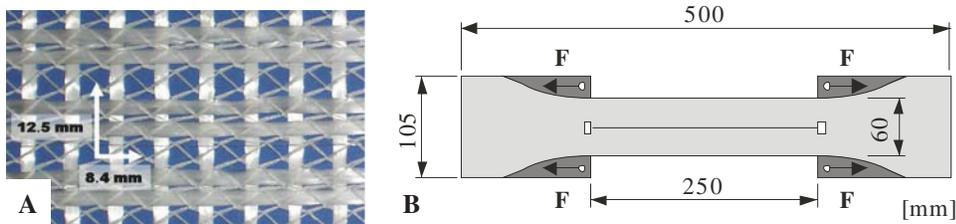
Fig. 3.1 – A) Applied AR-glass fabric manufactured at the Institut für Textiltechnik, RWTH Aachen University, Germany. B) Dumbbell tensile specimen with dimensions. (1 mm =  $3.937 \cdot 10^{-2}$  in.)
