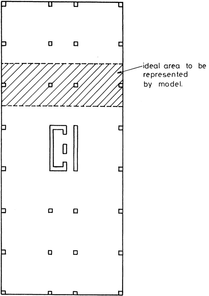
Fig. 1--Typical floor plan of a slab/column structure
