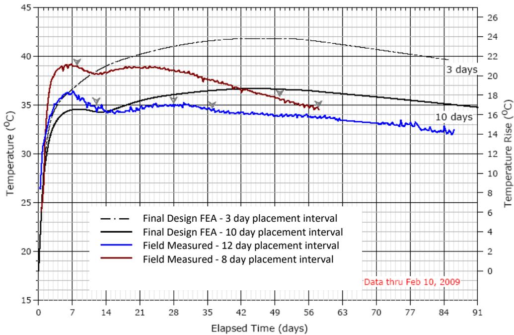
Figure 10 – Comparison of Measured and Computed Temperatures (Final Design Study)
