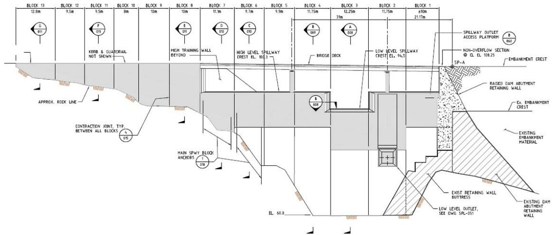
**Figure 3 – Upstream Elevation of Stage 3 Spillway Raise**
