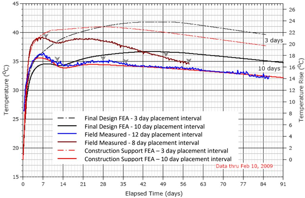
**Figure 12 – Comparison of Measured and Computed Temperatures (Final Design Study in Black, Construction Support Study in Red)**
