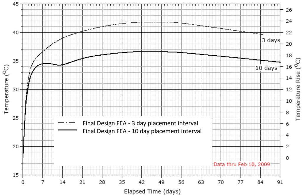
Figure 9 – Typical Computed Temperatures in Mass Concrete Lifts
