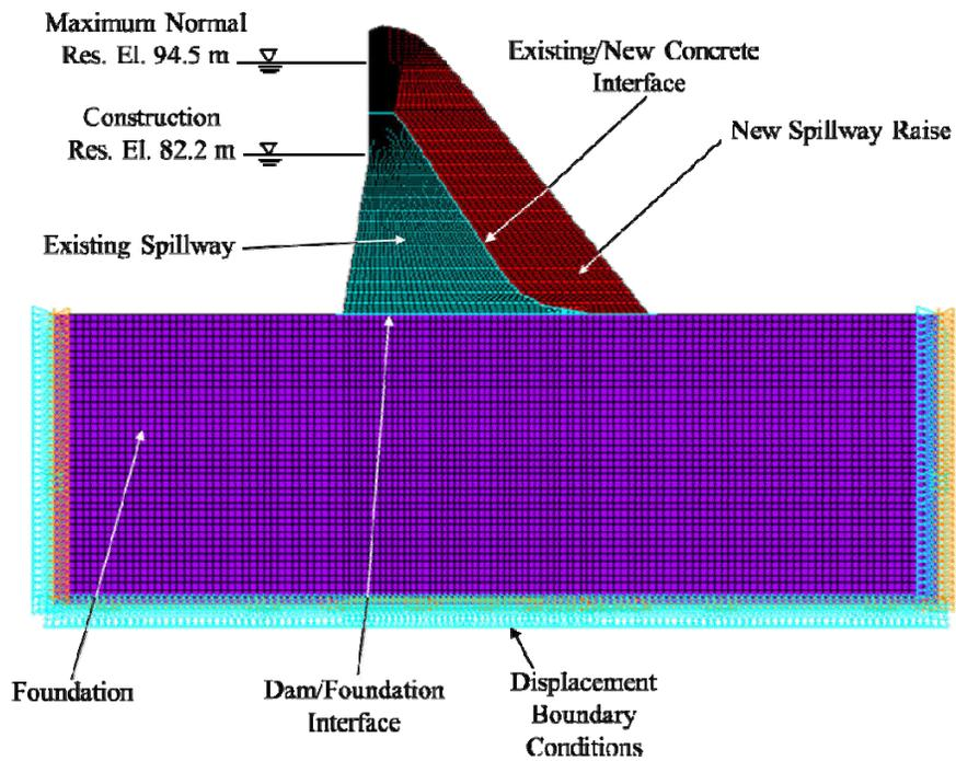
Figure 6 – FE Model of Spillway Maximum Section
