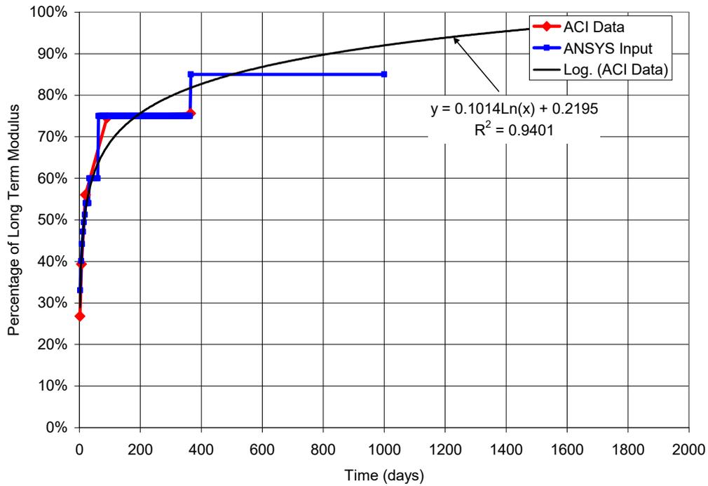
**Figure 13 – Variation of Modulus of Elasticity with Time**
