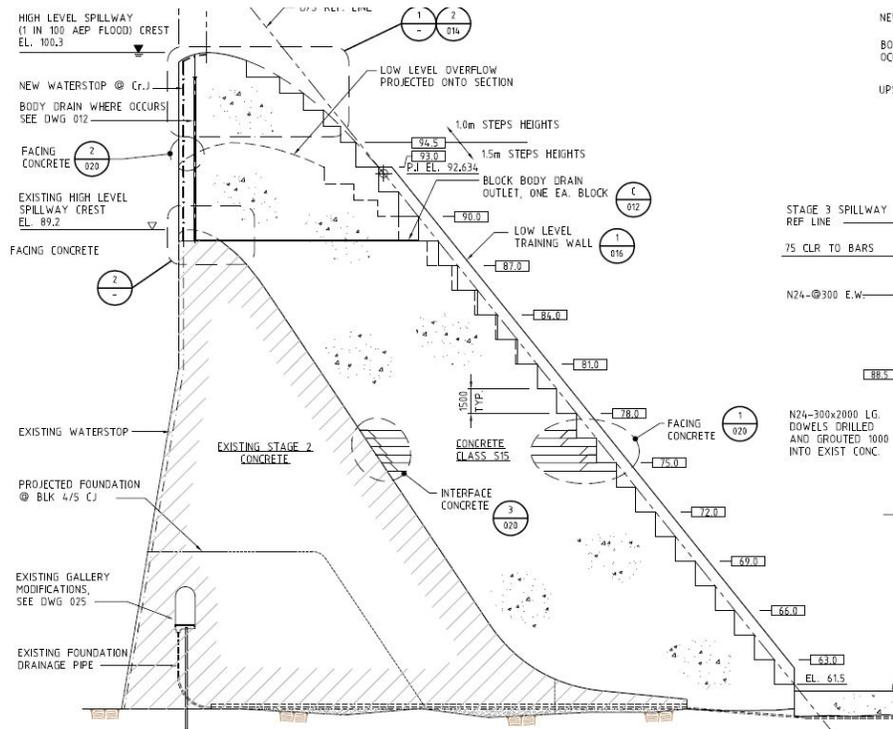
**Figure 4 – Stage 3 Spillway Raise High Level Spillway Monolith**
