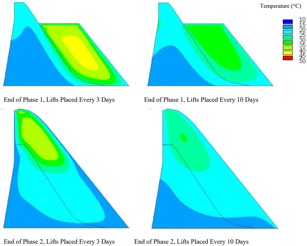
**Figure 11 – Temperatures Computed in Construction Support Studies**
