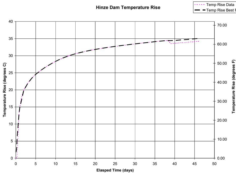
Figure 5 – Adiabatic Temperature Rise from Reclamation Tests
