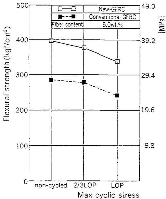
Fig. 10--Results of flexural fatigue test (flexural strength)
