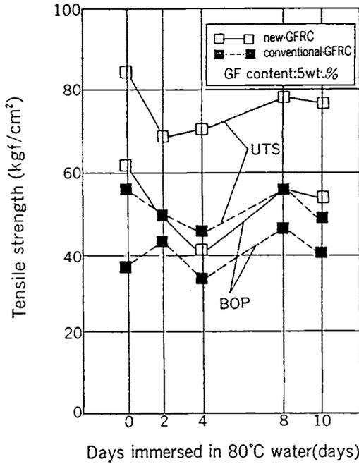
Fig. 6--Relation between days immersed in 80° C water and tensile strength of GFRC
