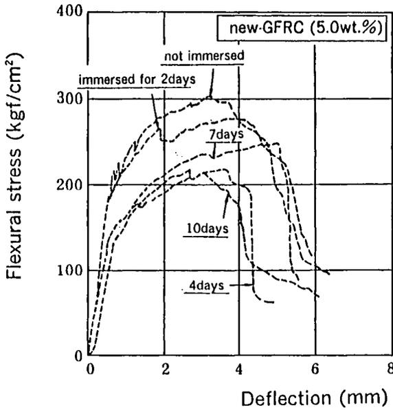
Fig. 5--Flexural stress-deflection curves for new-GFRC in 80° C water
