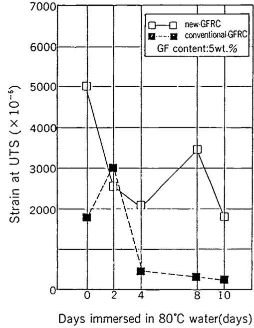
Fig. 7--Relation between days immersed in 80° C water and strain at UTS of GFRC
