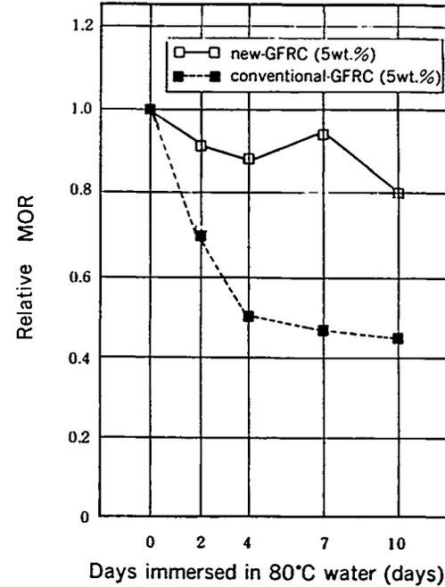
Fig. 3--Relation between days immersed in 80° C water and relative modulus of rupture of GFRC
