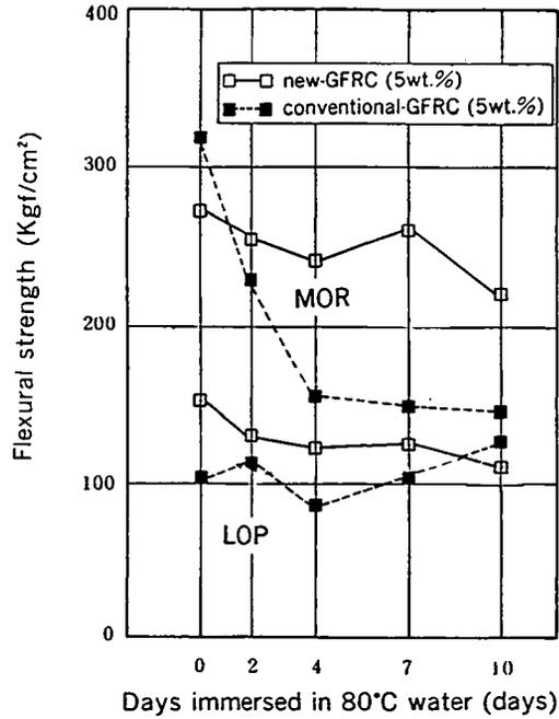
Fig. 2--Relation between days immersed in 80° C water and flexural strength of GFRC
