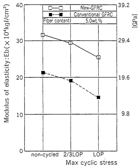
Fig. 11--Results of flexural fatigue test (modulus of elasticity)
