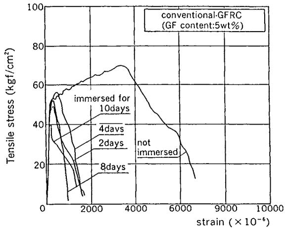
Fig. 9--Tensile stress-strain curves for conventional-GFRC immersed in 80° C water
