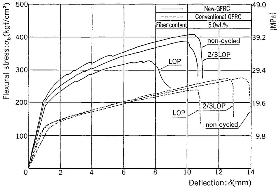
Fig. 12--Flexural stress-deflection curves
