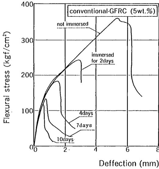
Fig. 4--Flexural stress-deflection curves for conventional-GFRC immersed in 80° C water
