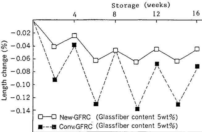
Fig. 14--Relation between drying at 20° C •30%RH / wetting at 20° C •90%RH cycle and length change
