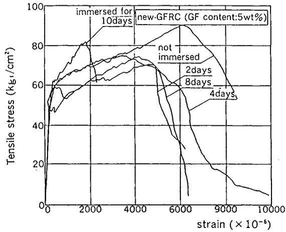
Fig. 8--Tensile stress-strain curves for new-GFRC immersed in 80° C water
