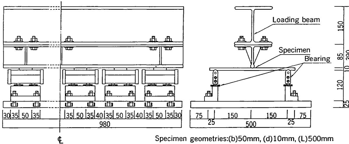
Fig. 1--Flexural fatigue testing method
