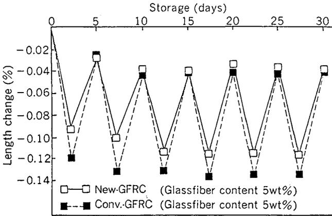
Fig. 13--Relation between drying at 70° C / wetting at 20° C cycle and length change
