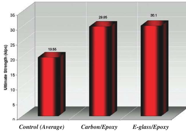
**Figure 14**—Strength Comparison between Strengthened and Unstrengthened (*As-Built*) Column-Tie Beam Joint Specimens.
