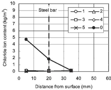
Fig.9 Chloride ion profiles in concrete
