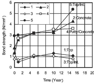
Fig. 7 Change in bond strength of surface coating materials with time
