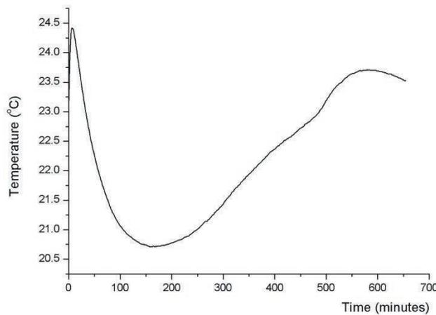
Figure 4 – Temperature change of w/c 0.5 cement paste obtained during UWR measurement (temperature ranges from 69 ~ 76 °F, conversion factor 1 °C = 1.8 °F (1.8×T<sub>c</sub> + 32))
