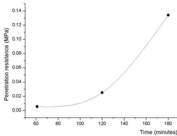
Figure 6 – Penetration resistance data of w/c 0.5 cement paste during first 3 hours (penetration resistance ranges from 0 to 20 psi, conversion factor 1 MPa = 145 psi)
