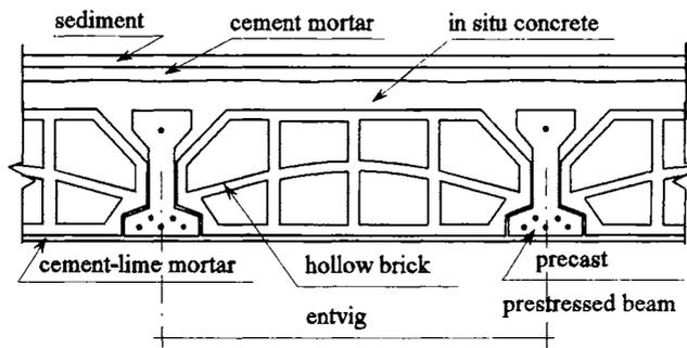
Fig. 1—Slab cross-section.
