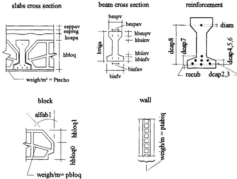
Fig. 3—Cross-section geometry and its variables.
