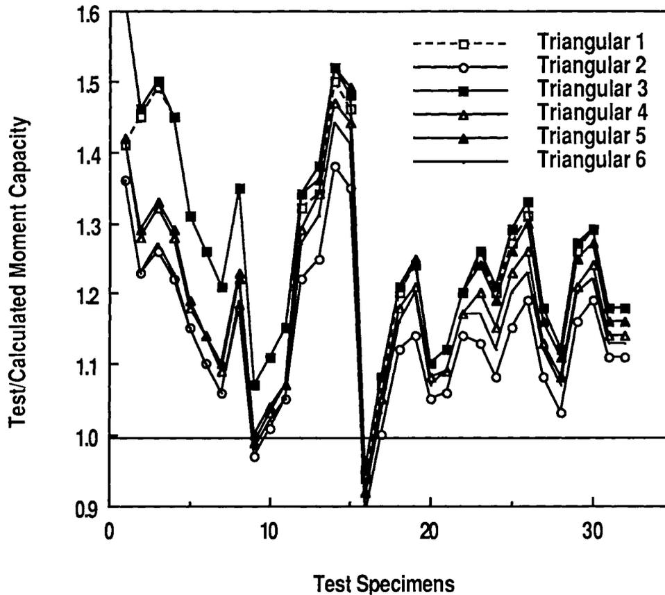
Fig. 7--Flexural strength prediction by triangular stress blocks
