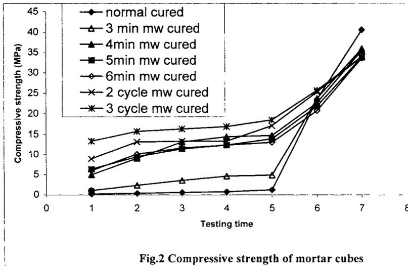
Fig.2 Compressive strength of mortar cubes
