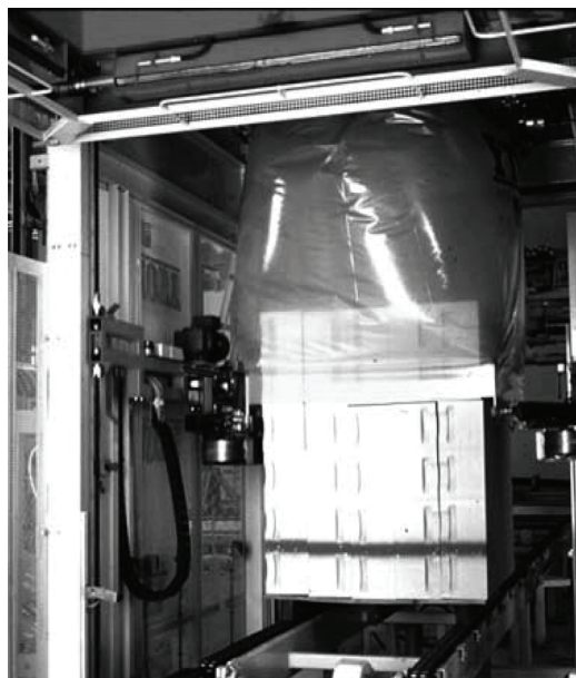
Fig. 3.5—Packaging of finished AAC units.
