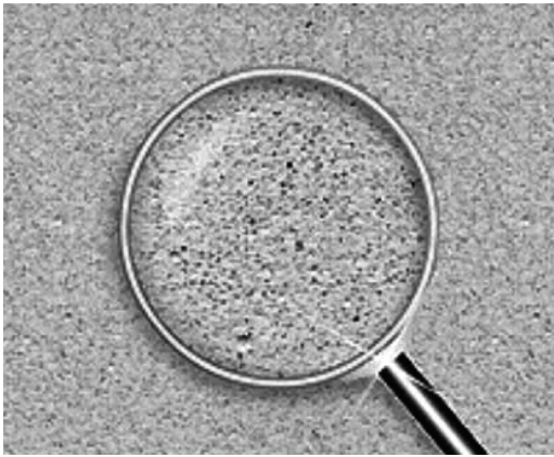
Fig. 1.1—Macroscopic cellular (void) structure of AAC.
