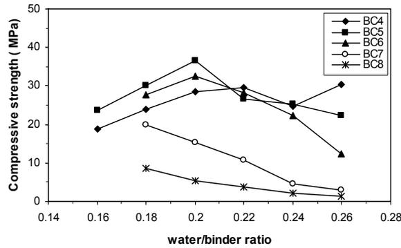
Figure 5—Influence of  $w/b$  loading on average compressive strength (1 MPa = 0.145 ksi)
