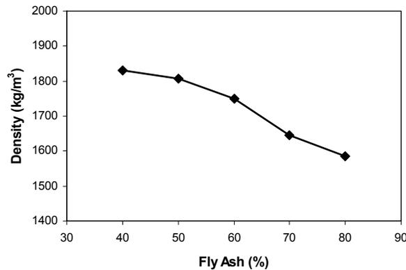
Figure 4 —Average density vs fly ash loading by mass of binder (1 kg/m<sup>3</sup>=1.685 lb/yd<sup>3</sup>)
