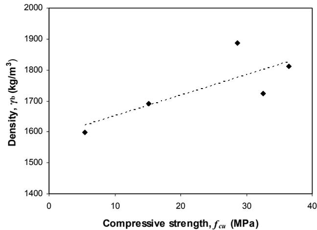
Figure 6 —Relationship between binder average compressive strength and average density (1 MPa = 0.145 ksi; 1 kg/m<sup>3</sup> = 1.6855 lbs/yd<sup>3</sup>)
