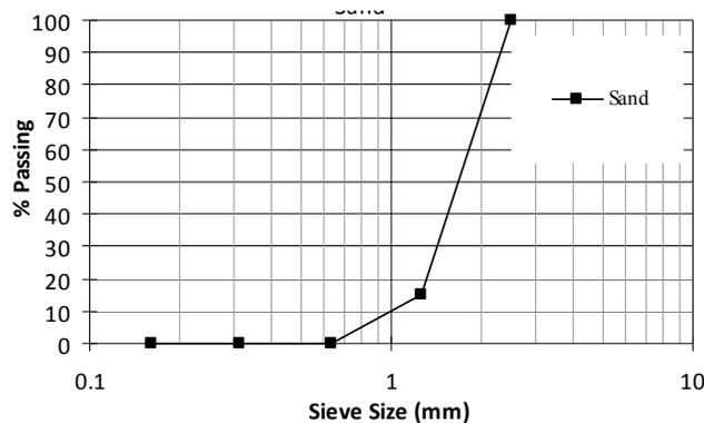
Figure 1—Particle size distribution of sand (1 mm = 0.039 in.)
