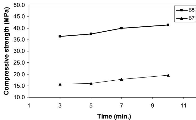
Figure 3—Influence of mixing time on average 7-day compressive strength (1 MPa = 0.145 ksi)
