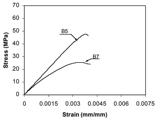
Figure 8—Compressive stress-strain response of binders B5 and B7 (1 MPa = 0.145 ksi)
