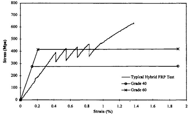
Fig. 2—Stress-strain curves of hybrid FRP reinforcing bars versus Grade 30/60 reinforcing bars.
