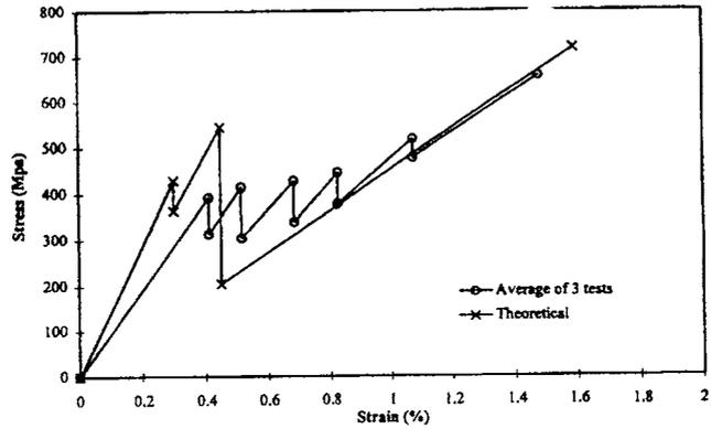
Fig. 1—Theoretical versus experimental stress-strain curves of hybrid FRP reinforcing bars.
