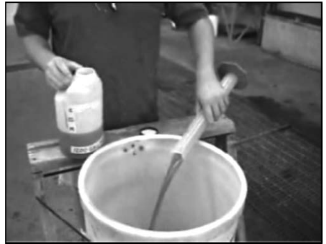
Fig. 2.1—Diluting foam concentrate in water (click on picture to view video).
