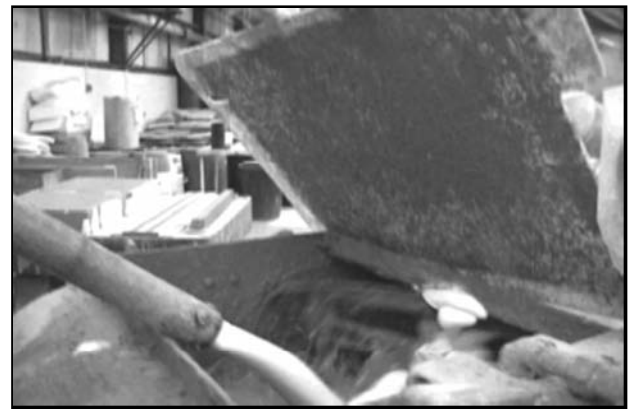
Fig. 2.2—Metering preformed foam into cement-water slurry (click on picture to view video).
