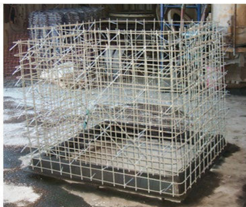
Fig. 2—A complete GFRP cage before concrete casting
