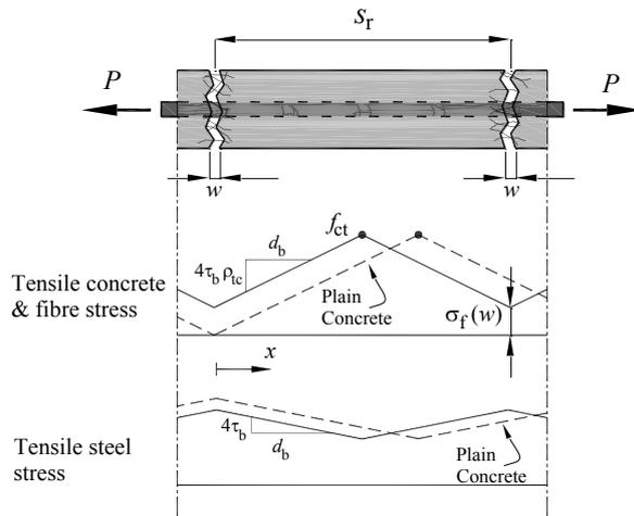
Figure 4: Crack spacing representation using TCM
