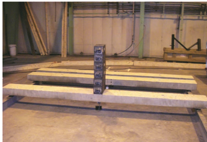
Fig. 4—Setup for live load.
