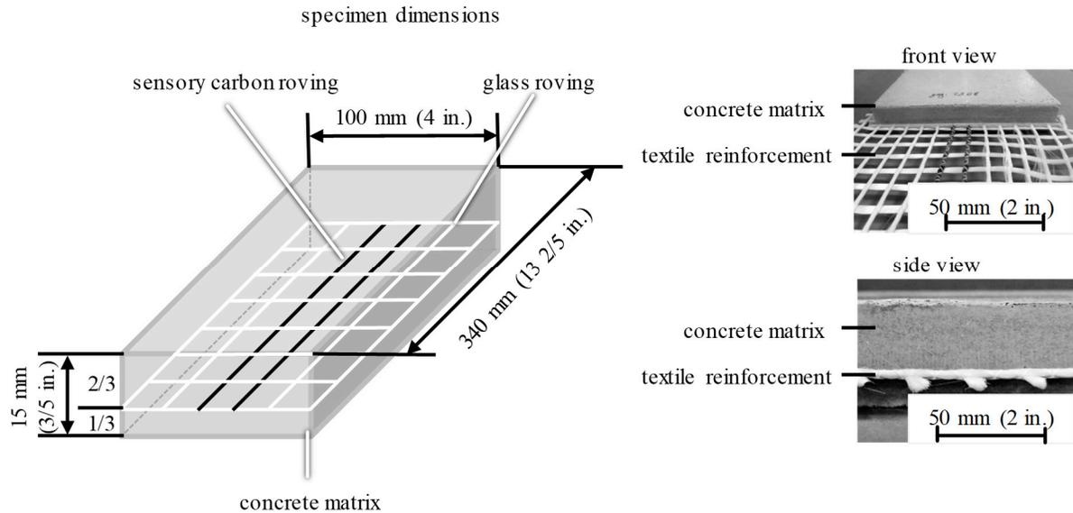
**Figure 1** – Specimen dimensions for the four-point-bending tests
