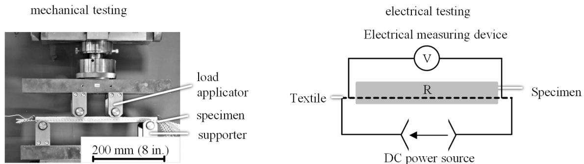
**Figure 2** – Set-up of the four-point bending test (left) and circuit diagram for the electrical measurements (right)
