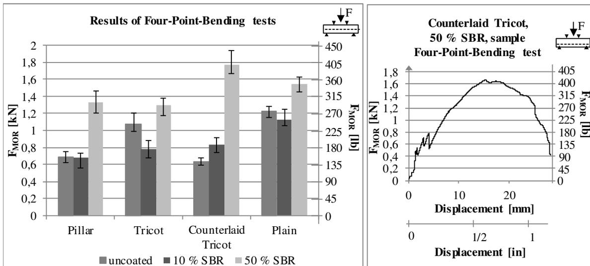
**Figure 3** – Mechanical results of the four-point-bending tests and the representative load response for counterlaid tricot, 50 % SBR coating
