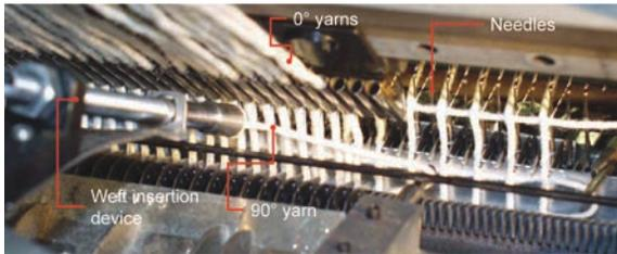
Fig. 5—Detail of warp knitting area with weft insertion yarns.
