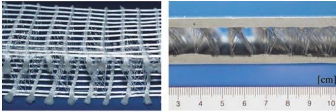
Fig. 3—Spacer fabric: a) Type A; and b) Type A with thin walled concrete layers on both sides.
