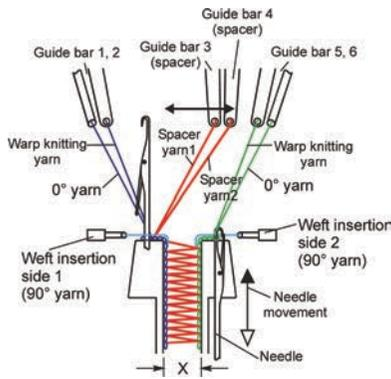
Fig. 4—Schematic cross section of warp knitting elements.
