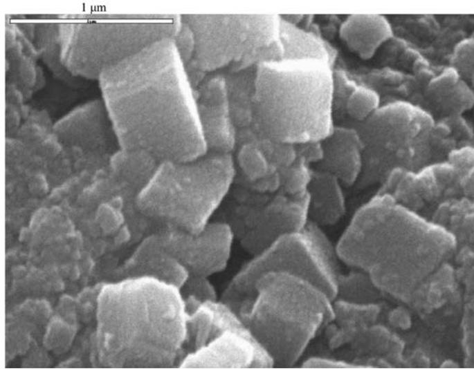
Fig. 9—Sample containing 150 nm silicon dioxide at 40,000× magnification.
