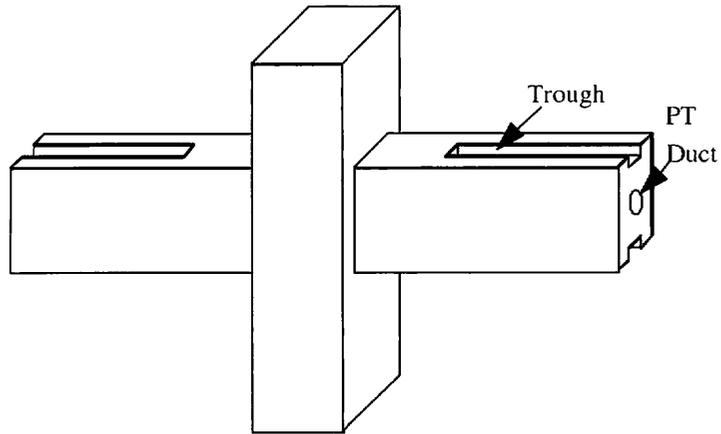
Figure 5 Phase IV B Specimens – Beams with Troughs and Central PT.
