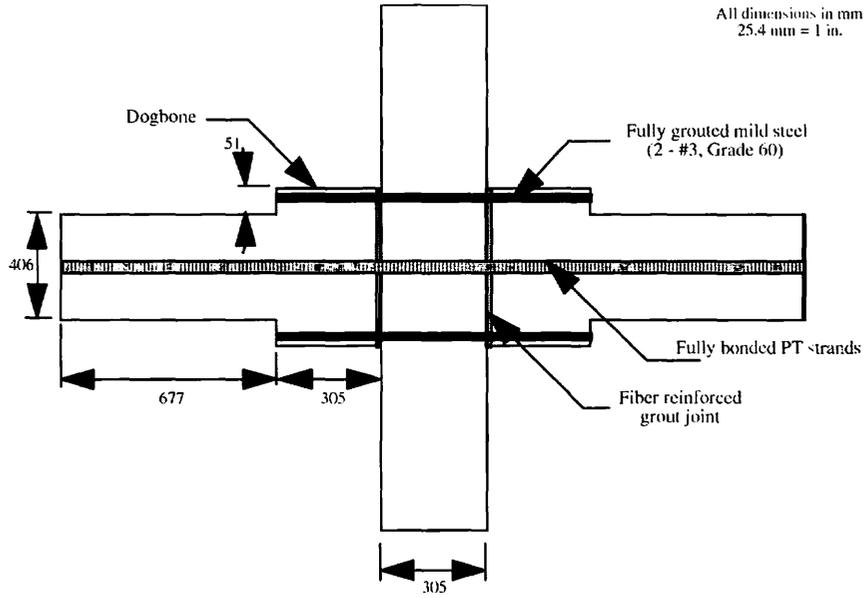
Figure 3a Specimen I-P-Z4 and K-P-Z4.
