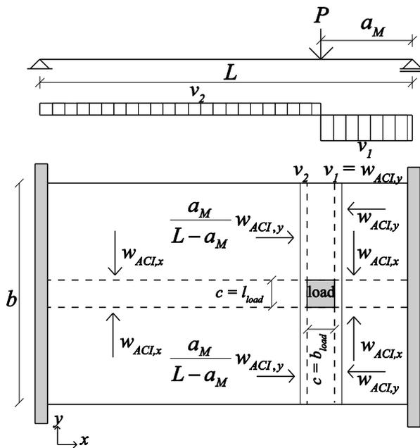
Figure 3: Overview of loads on strips in *x*- and *y*-direction and implications of static equilibrium.
