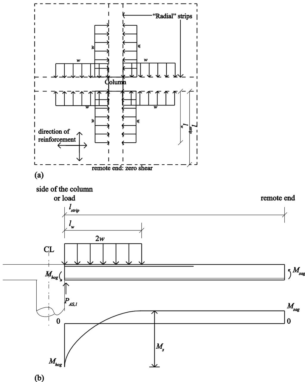
Figure 2: Overview of the Bond Model for concentric punching shear: (a) layout of the slab, divided in quadrants and strips; (b) loading situation on strip and resulting moment diagram (Alexander and Simmonds, 1992).
