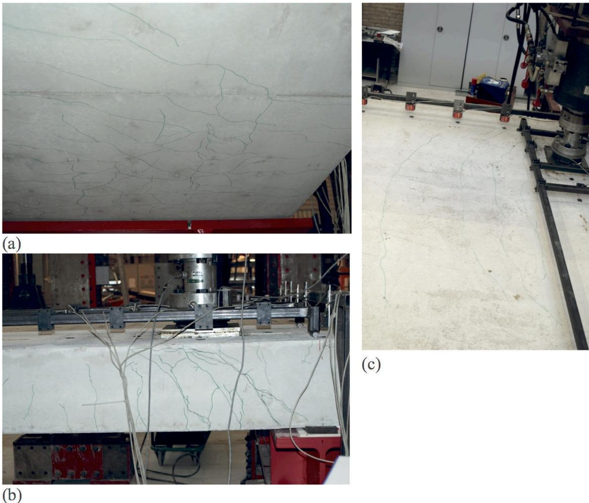
Figure 1: Observed cracking after failure of slab S6 in experiment S6T4 (Lantsoght *et al.*, 2013b): (a) combination of one-way shear (inclined cracks on the bottom face), torsional distress at the edge and flexural distress represented by longitudinal and transverse cracks; (b) one-way shear failure crack at the edge; (c): two-way shear cracks on the top face of the slab.
