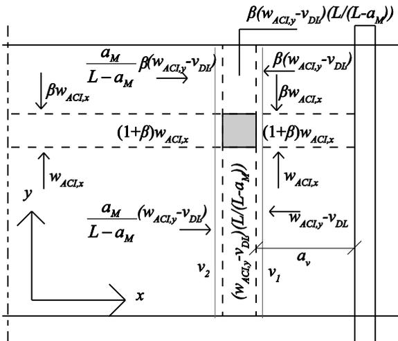
Figure 4: Overview of loads on strips in  $x$ - and  $y$ -direction and implications of static equilibrium, including reduction of self-weight and effect of torsion.
