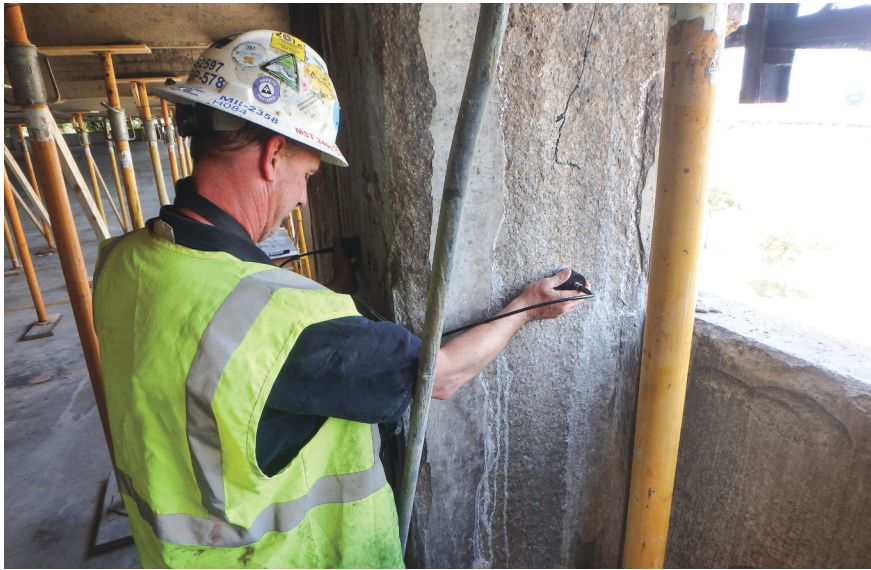
Fig. 5—Nondestructive testing performed at damaged column
