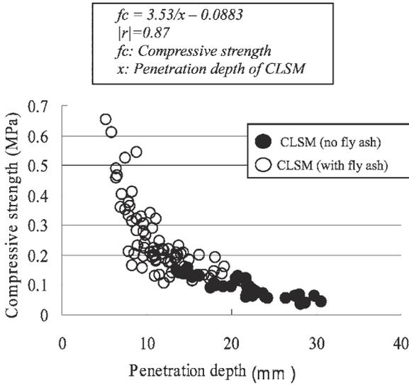
Figure 3 – Relationship between compressive strength and penetration depth.
