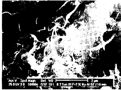
Fig. 6 Paste with 2 % accelerator (no SP, \times 16000 ), 10 minutes hydration
