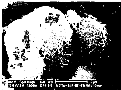
Fig. 8 Paste with 2 % accelerator and 2 % SP ( \times 16000 ), 10 minutes hydration
