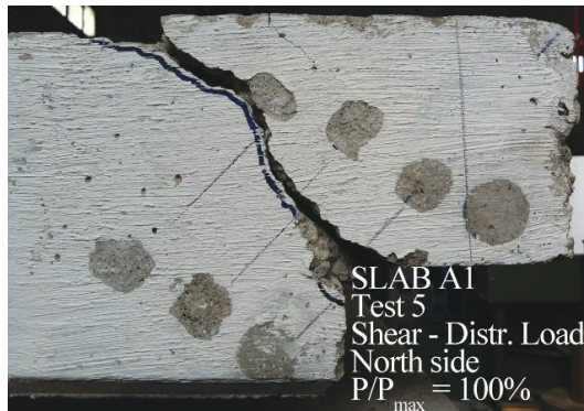
Figure 9 - Slab A1 with hooks and bent-up bars: shear Test 5, distributed load, P_u = 401 \text{ kN} [90 kips].
