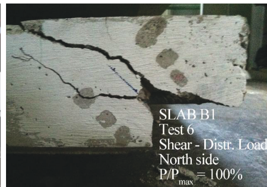
Figure 10 - Slab B1 with straight bars: shear Test 6, distributed load, P_u = 172 \text{ kN} [39 kips].
