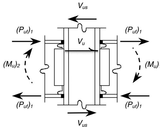
Note: shear forces in beams and moments and axial forces in column omitted for clarity.
