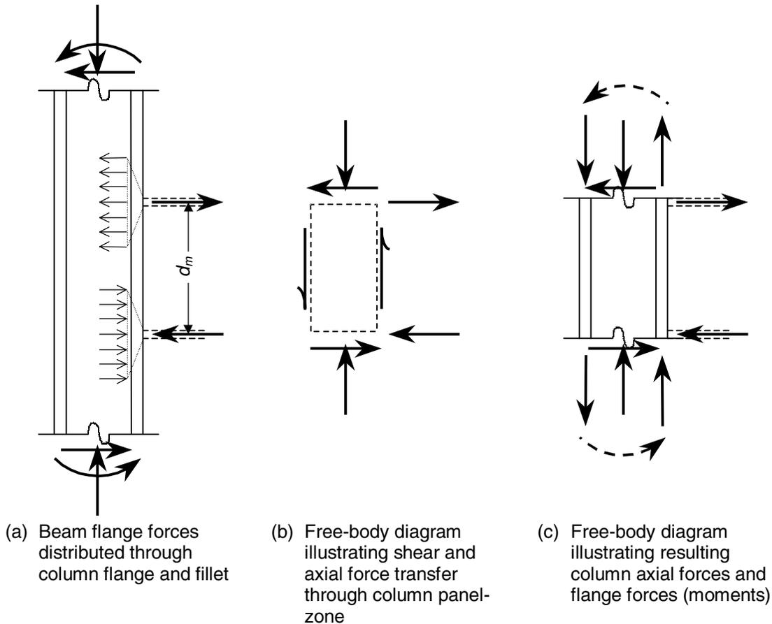
Note: beam shear and axial force (if any) omitted for clarity.
