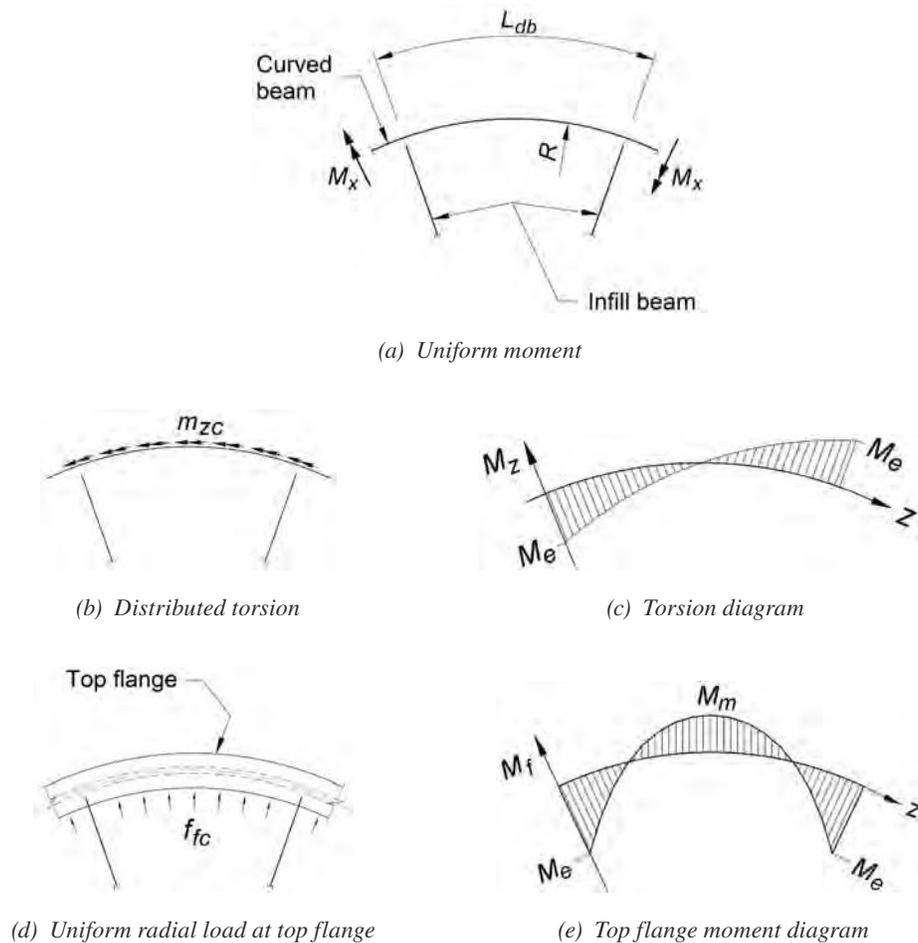
Fig. 7-2. Curved beam continuous across torsional supports.
