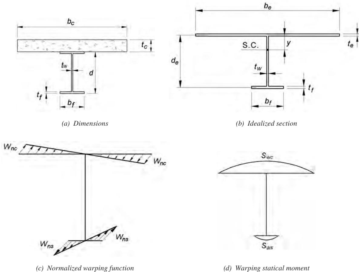
Fig. 7-5. Torsional properties of a composite beam.
