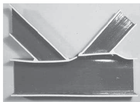
(b) Longitudinal cross-section through an HSS K-connection at ultimate load.
