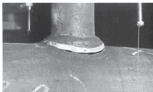
(b) Round HSS T-connection at ultimate load.
