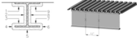
Fig. IX.2 SFRM Thickness Measurement Locations at Beams
